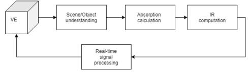
Fig. 1: a diagram showing a design for the system proposed. a method for object/scene understanding is applied in order to extract information that would be used to calculate sound absorption of surfaces and objects. As a result, impulse responses would be computed and integrated to the sound signal through real-time algorithms.
