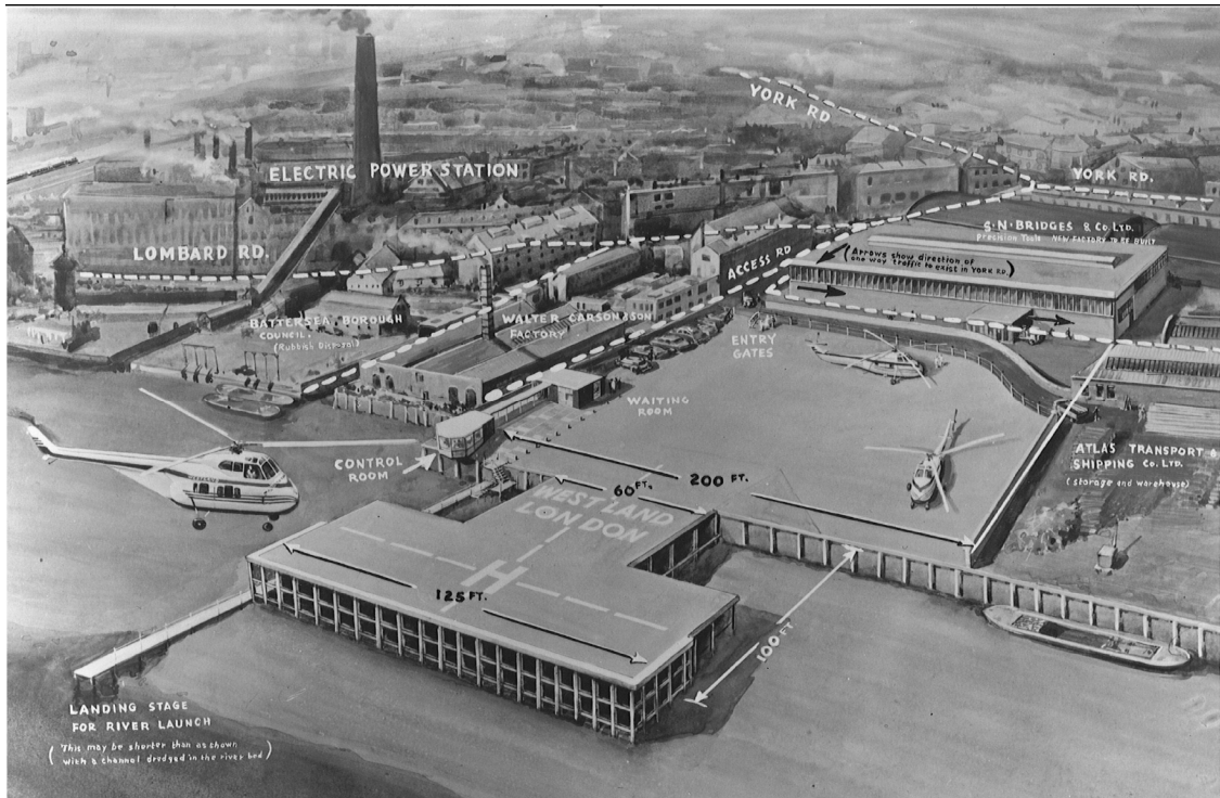
Figure 3. The Westland Heliport at Battersea shown in an explanatory drawing from its planning in the late 1950s (Helicopter Foundation International, historical archive, < http://archives.rotor.com >).
